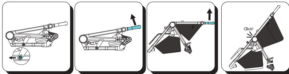
3. Assembling/Disassembling of the bumper
