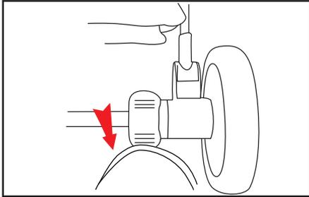
Brake adjust: as shown by arrow, step on brake lever backward to be in the braking state.
