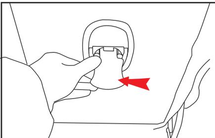
Adjusting the backrest: Press the "Adjusting button" and pull it backward to release the backrest.
