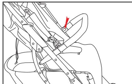
Press the button shown by the arrow to open or remove the armrest.
