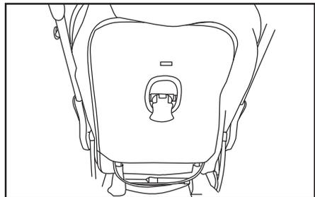
The Angle of the backrest can be adjusted upward by pushing the backrest directly.
