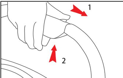
Sliding the button "1" towards left, press down the button 2 to unlock stroller.
