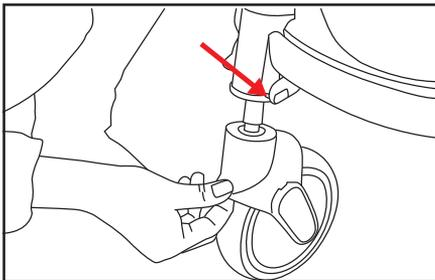
Disassembling front wheel: Press the showed white button can remove the front wheels.
