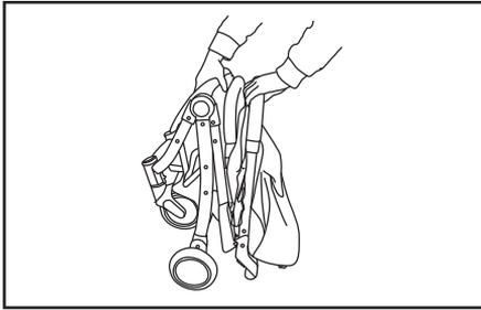
Using hook to lock the folded stroller
