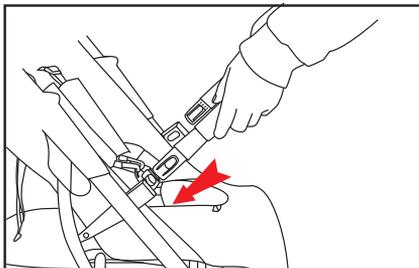
As indicated by the arrows, insert the front bumper into the slot, hear "click" means OK.
