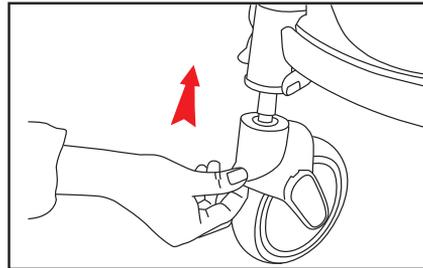
Front wheels: Insert the front wheel axle into the corresponding hole.
