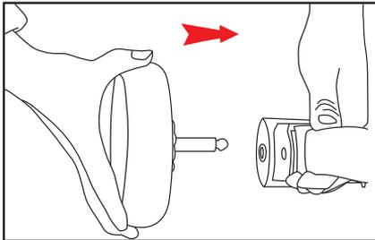
Rear wheels: Insert the rear wheel axle into the corresponding hole.
