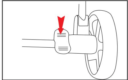
Brake adjust: as shown by arrow, step on brake lever forward to unlock.
