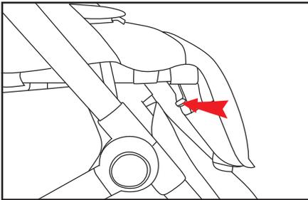
Footrest adjusting: Press arrow pointer buttons to adjust, release buttons to make the footrest pedal down mode.
