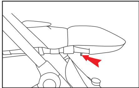
Press the arrow pointer button, pull up the footrest adjustor, this figure is footrest up mode.
